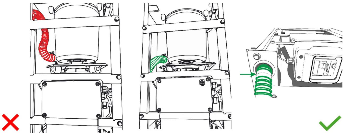
Install a **PROTECTIVE PLATE** underneath the dryer using the same bolts from removed transit bar. The protective plate must be always in **OPERATION MODE**.
